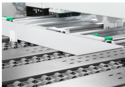
Automatic alignment of the board. No further striking or alignment. Fast bending sequences, high productivity.
