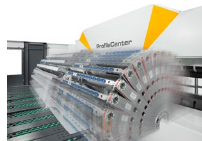
Automatic bending with fast cycle times. The workpiece does not have to be positioned at the stops during bending process.
