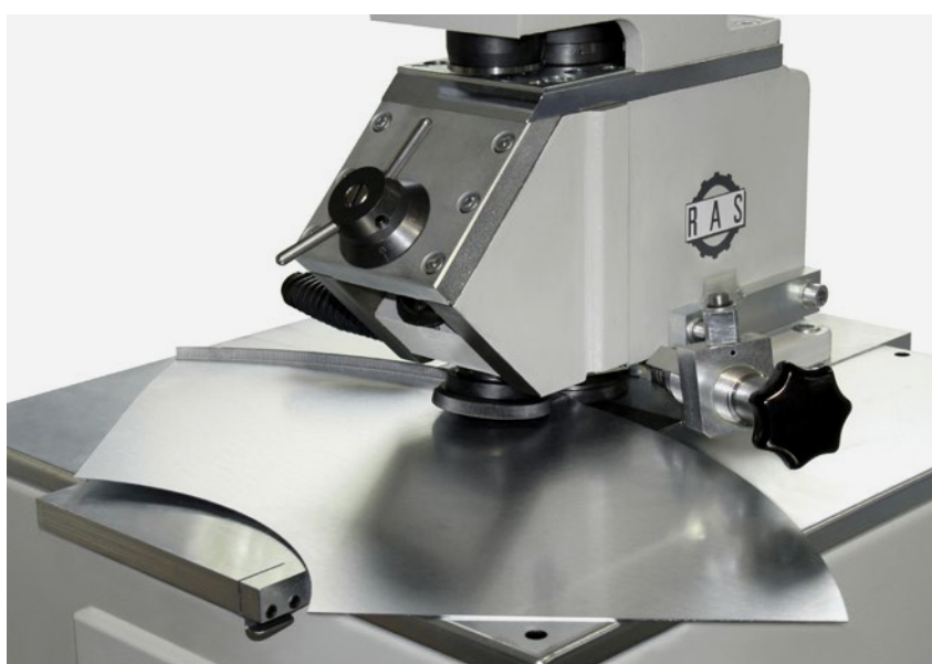
Automatic sheet guide system
