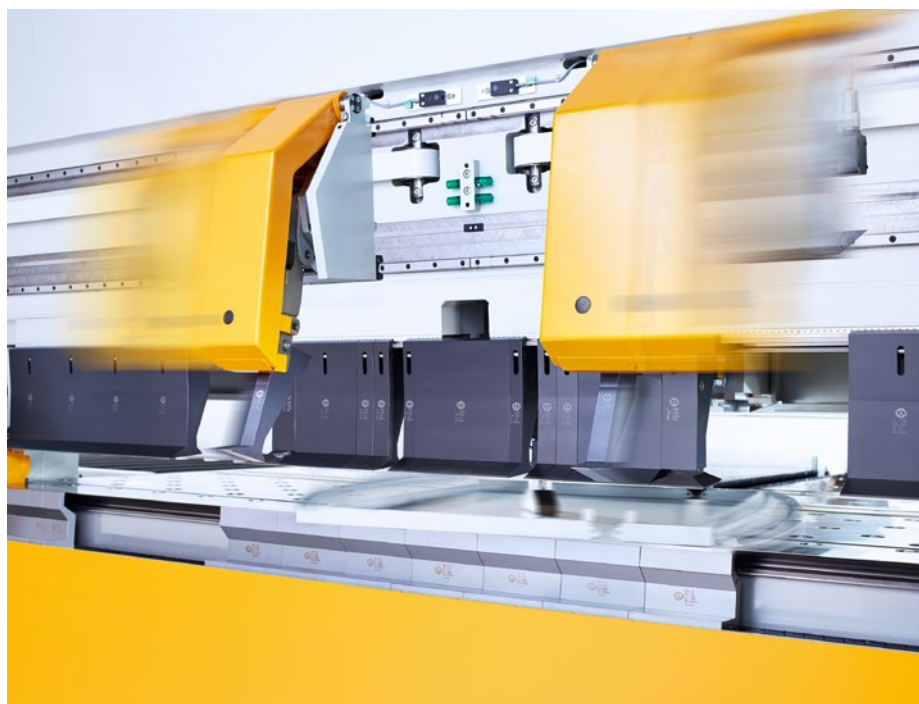
Fully automatic bending sequences: positioning, rotation, bending, and tool change.
