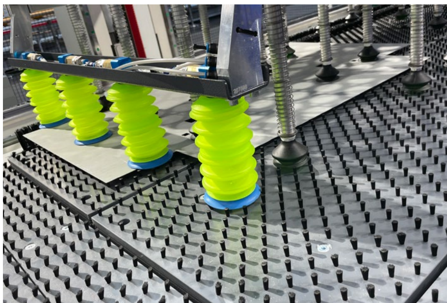
Loading system for automatic feeding of blanks from a stack of sheets with sorted and edge-precisely stacked sheets
