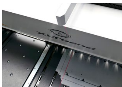
The laser beam of the Virtual Navigator (ViN) shows the exact part loading position.
