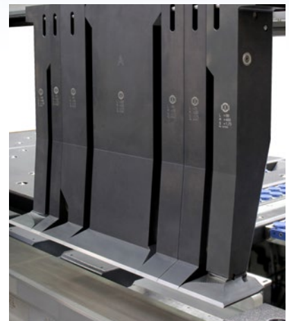
Upper beam tools as tall as 600 mm
