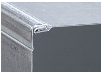
Improved seaming accuracy also results in a reduced distortion of the duct cross-section.
