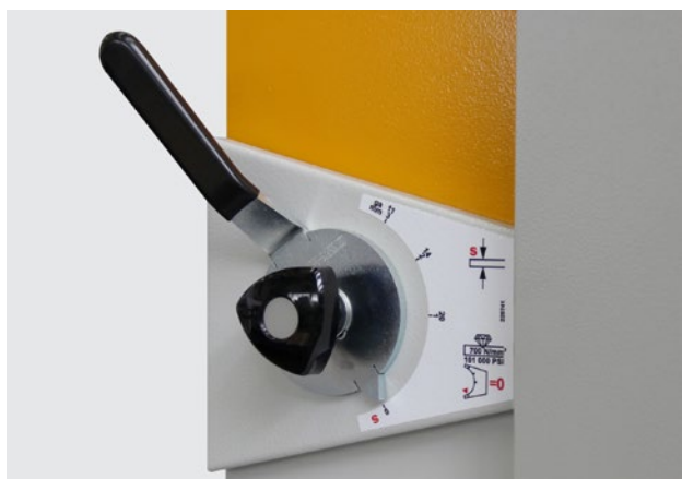
Lever for the cutting gap adjustment on the PRIMEcut.
